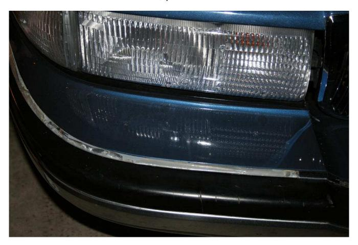
First you must remove the old trim. It's held on with adhesive tape. Use a small flat object to get started. Flat blade screwdrivers will work but you must be cautious not to gouge your bumper cover. Plastic razor blades (see your local body shop supply for these) or a putty knife also work well.
