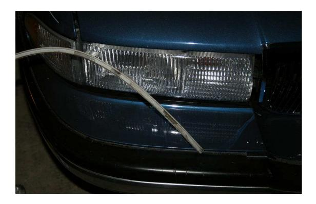
Now you need to remove all of the remaining adhesive tape. A plastic scraper or any flat tool will work here too. Again, be careful not to scrape your bumper cover. Placing the car in the sun for a bit will help to soften the tape.
